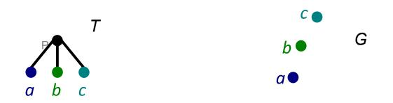
**cograph** G = graph without induced  $P_4$ graph built by series composition (**s**eries operation) and disjoint union (**p**arallel operation)  $\rightarrow$  cotree T
