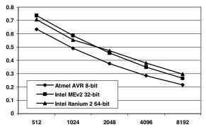
Figure 2: Ratio of Runtime: Modified Barrett / Montgomery  $\left(\frac{T_B}{T_M}\right)$  vs. Modulus Length (in bits) on three architectures.
